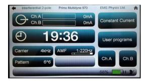
Interferential 2-pole therapy is similar to Interferential 4-pole except that the two medium frequencies are added together in the stimulator itself and applied to the treatment site through a single pair of electrodes. Two separate outputs A and B are available with independent level controls.
