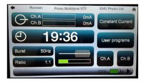
Russian stimulation therapy consists of a 2.5kHz medium frequency which is modulated on and off in bursts that can be set anywhere between 1 and 100Hz. An overall surge envelope can also be applied with variable work and rest periods.
